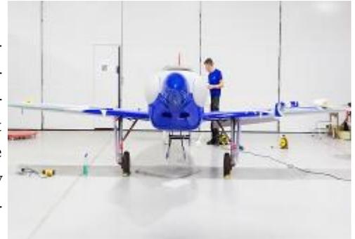
That's thanks to "the world's most energy-dense flying battery pack," according to Rolls Royce. The aircraft has three batteries powering three motors that will deliver 750kW to spin the propellers. Each 72 kilowatt-hour battery pack weighs 450kg and has 6,000 densely packed lithium-ion cells.
