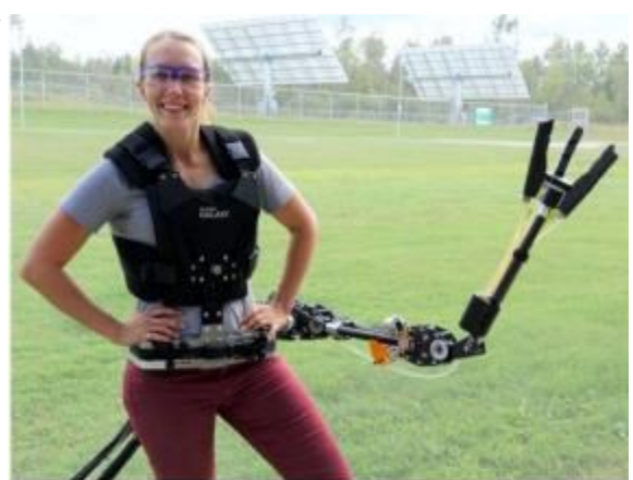
Photo: Université de Sherbrooke Researchers at the Université de Sherbrooke in Canada developed a waist-mounted hydraulic arm that can help you with all kinds of tasks.
